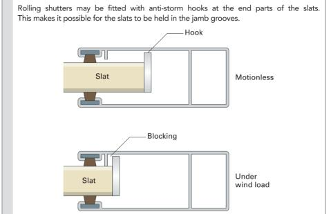
Figure 16: Example of an anti-storm hook
