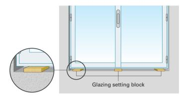
Figure 10: Example of shimming
