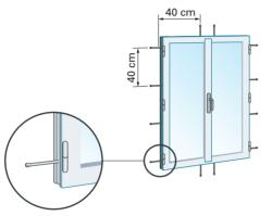
Figure 9: Principle for distance between fasteners
