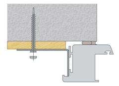
Figure 5: Example of bracket attachment
