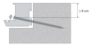
Figure 7: Example of fastening using "concrete screws"
