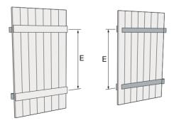
Figure 13: Traditional shutter with reinforcements
