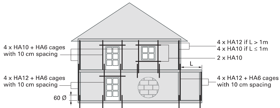
Figure 19: Example of vertical tie beam arrangement
