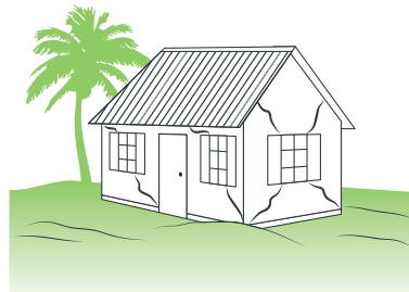
Figure 17: Cracks in solid walls (earthquake)
